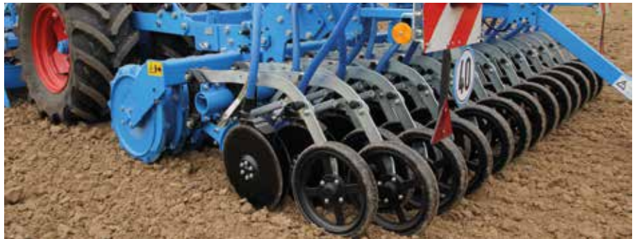
Maintenance free OptiDisc double disc coulters
